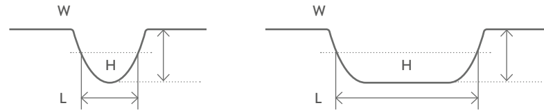
Minimum die roll cavity dimensions (mm)
